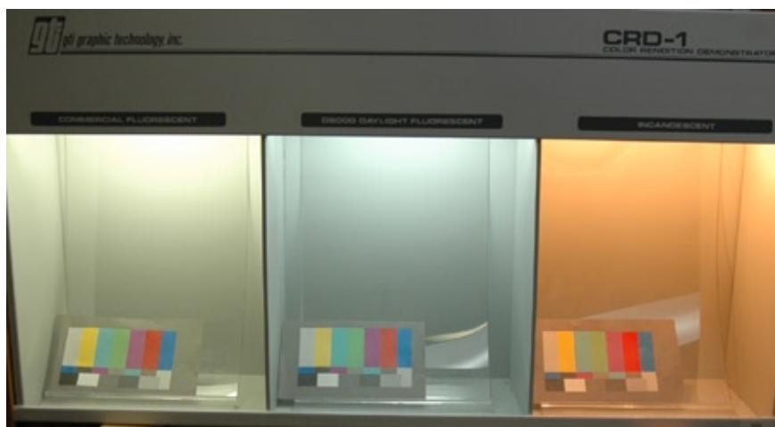
Fig. 1: Identical hardcopy prints under three different light sources [left: office illumination – „Cool white fluorescent“, middle: daylight simulator D50 according ISO 3664 [1], right: tungsten source].
